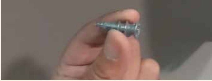
The Zip-It/Tornado anchor is a one-piece self drilling anchor designed specifically for use in gypsum wallboard.
